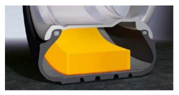
A special polyurethane foam, attached to the inner surface of the tire tread, cushions the road, providing a guieter driving experience.
