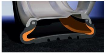
When a puncture occurs with a standard tire, the sidewall can become crushed between the rim and the road causing a potentially dangerous situation. The reinforced sidewall in the self supporting runflat tire prevents this from happening.
