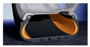
A self-supporting reinforced sidewall offers additional fortification, preventing the sidewall from being crushed between the rim and the road in the case of tire damage.
